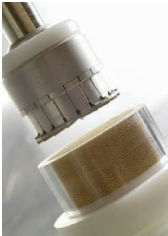
FIGURE 2. Shear-cell testing is a valuable technique for hopper design and, more generally, for assessing the performance of powders under conditions of moderate to high stress
