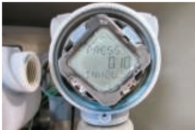
FIGURE 2. This image shows a cold-temperature qualification test for a pressure transmitter whose LCD is clearly readable at a temperature of -40^{\circ}\text{C}
