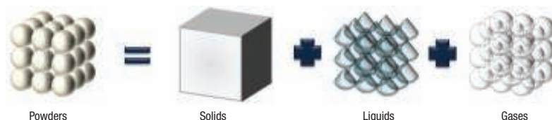
FIGURE 1. Powders are bulk assemblies consisting of solids, liquids and gases. Interactions between all three of these phases determine the bulk powder behavior
