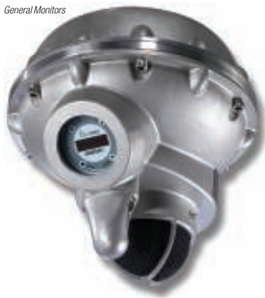
FIGURE 4. Ultrasonic gas leak detectors use acoustic technology to swiftly detect outdoor gas leaks by sensing the distinct high-frequency ultrasound emitted by high-pressure gas leaks, allowing faster response times
