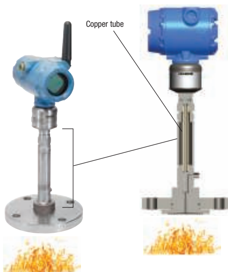
FIGURE 7. A thermally optimized, single-oil seal system eliminates the need for heat tracing, without compromising measurement responsiveness, for close-coupled, gage pressure applications
