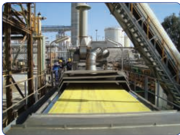
A Berndorf Band steel belt made from corrosion-resistant NICRO 85 in use for sulfur recovery at a refinery in Spain
