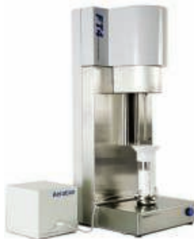
FIGURE 3. Powder testers that offer multifaceted powder characterization, including dynamic testing, have a proven track record of supplying valuable information for process-related studies
