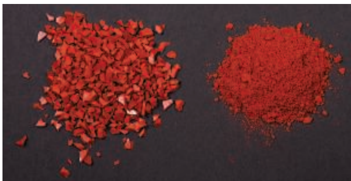
FIGURE 2. Cryogenic grinding allows even difficult materials like silicones to be reduced to a uniformly fine particle size
