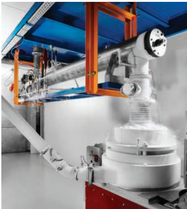
FIGURE 5. This ultrafine grinding mill uses liquid nitrogen for refrigeration
